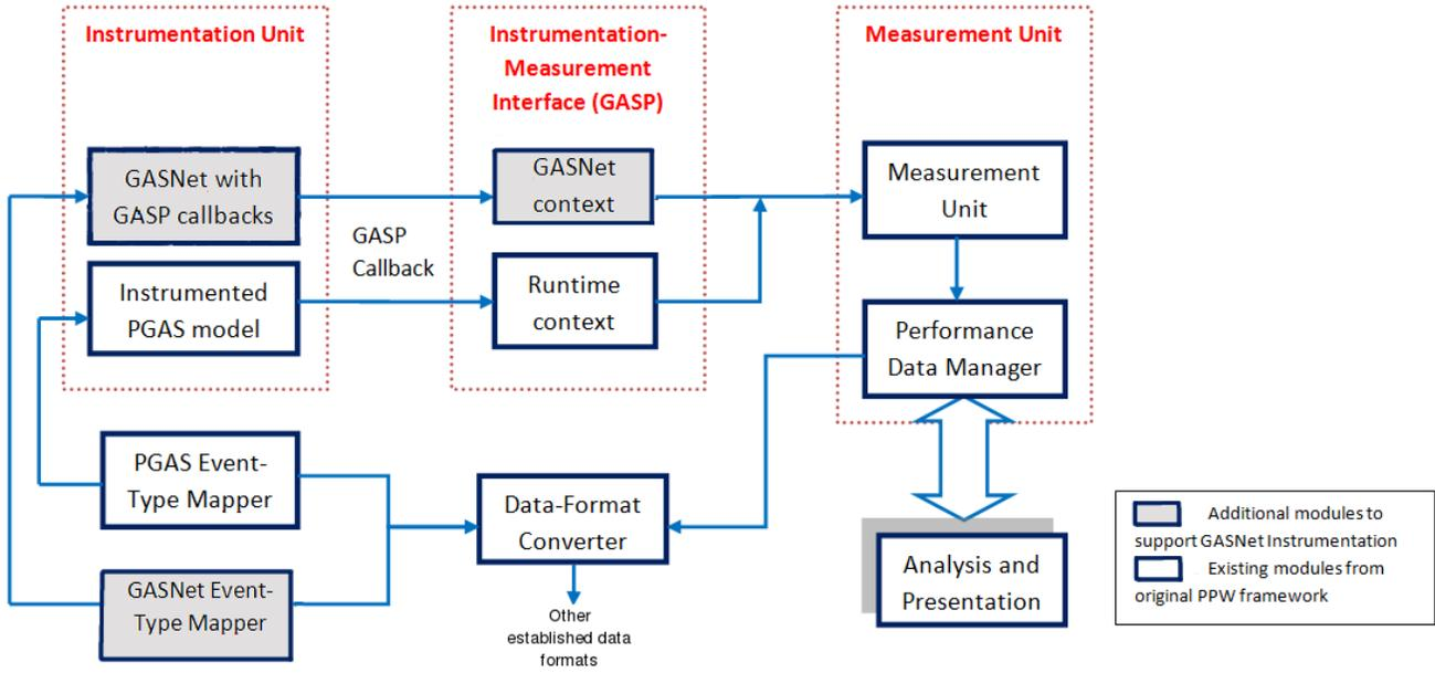
Figure 2. PPW framework to support GASNet instrumentation
