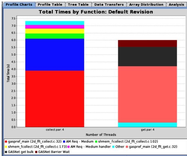
**Figure 8.** Snapshot showing time spent on different events in 2 different implementations of 2D-FFT
